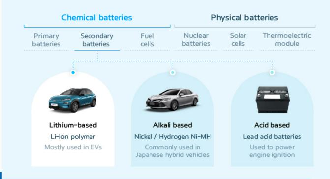
EVs source power from lithium-ion polymer batteries that are high density, light weight and satisfy excellent charge/discharge efficiency.
